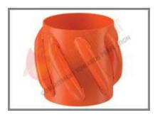
SledgeHammer's Solid Heavy duty Spirolizer are specially designed for extra heavy load in highly deviated Horizontal well and for use with Liner Hangers. The heavy steel construction is highly effective as compare to other alloy. Wide symmetrical Spiral fins are welded to the one piece rolled formed Sleeve under required temperature and condition with extra low Hydrogen coated Electrodes, which assures ultimate strength and uniformity in every weld.
